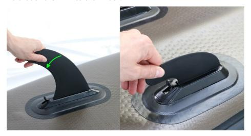
Lock the fin with the quick release lever.
